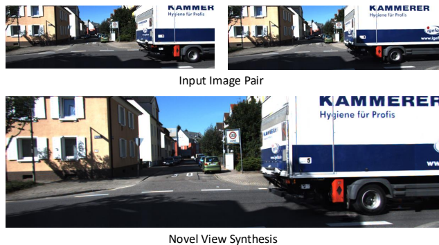
Figure 1. Dynamic Gaussian Splatting from An Unposed Image Pair. Given two images captured at distinct moments with unknown poses in a dynamic environment, our method can fit dynamic Gaussian splatting and then synthesize a new image from a novel viewpoint at a different time.
